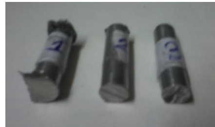
Fig.1 Samples of developed composite after wear
