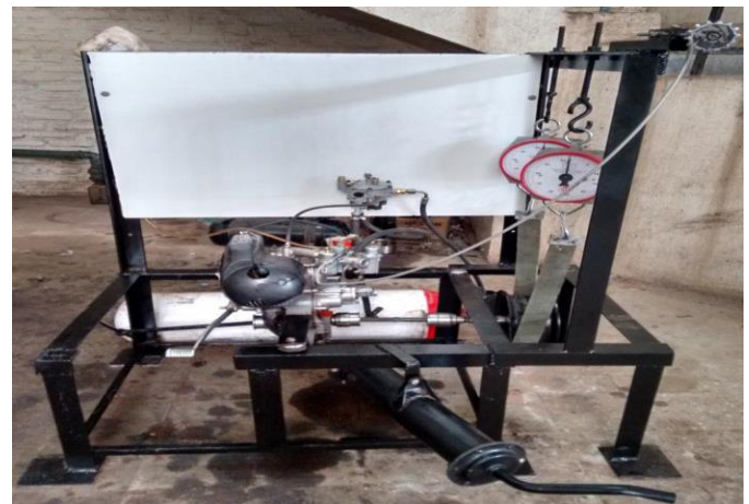
Fig.1 Two stroke single cylinder petrol engine test rig with rope brake Dynamometer
