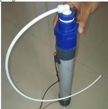
Fig. 2.3 Hydrogen production unit
