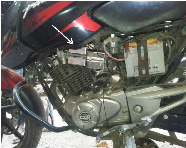
Fig.3. Location of the magnet at bike fuel line
