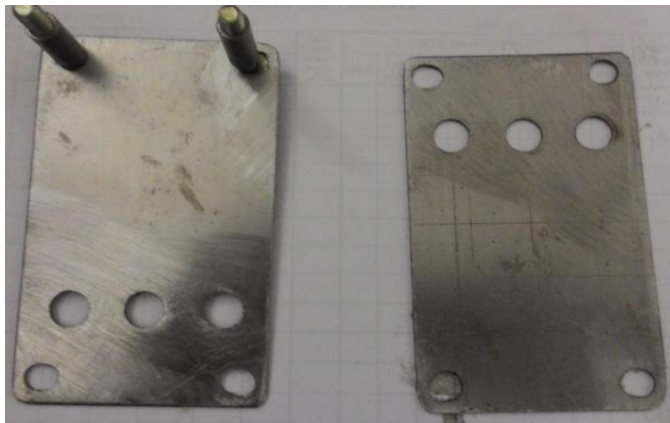
Fig. 4 Baffle Type 1 restrictor plate
