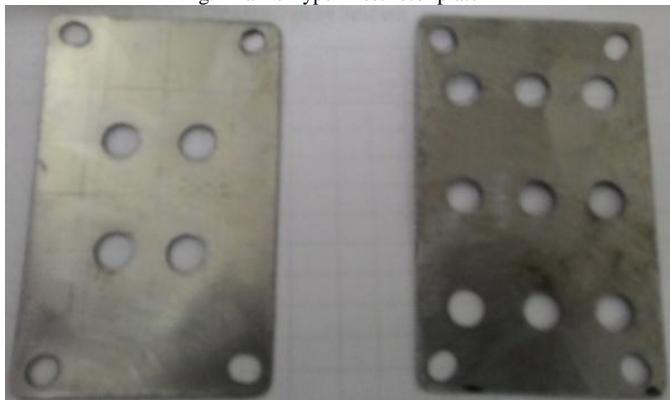
Fig. 5 Baffle Type 2 restrictor plate
