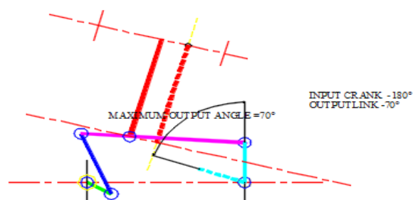
Figure 8 Input Crank at 180°, output crank at 70°
