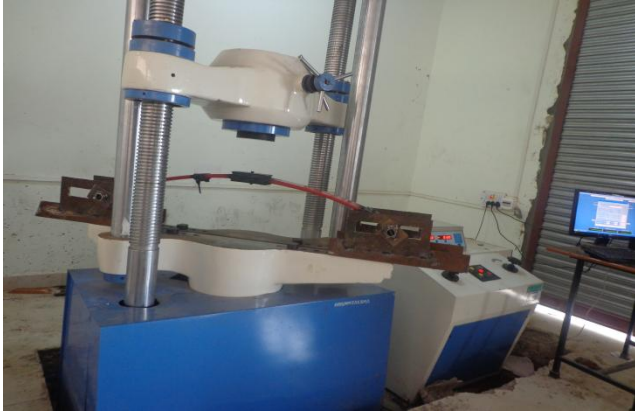
Fig.10. Test set-up on Universal Testing Machine.
