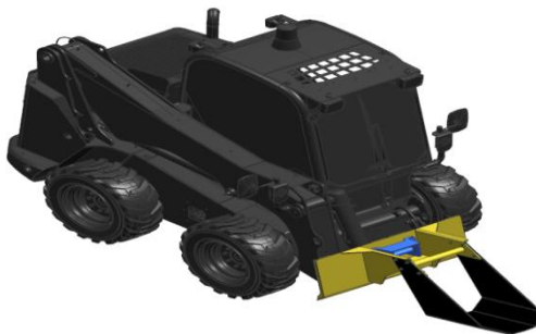
Figure 1 SKID STEER machine with digger attachment
