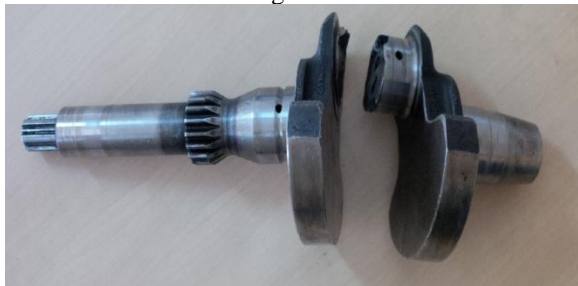
Fig. 1 Final failure On fillet of crankshaft
