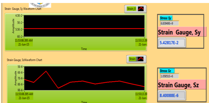
Fig.15 Screen shot showing the stress and strain readings at 0.2mm cut.
