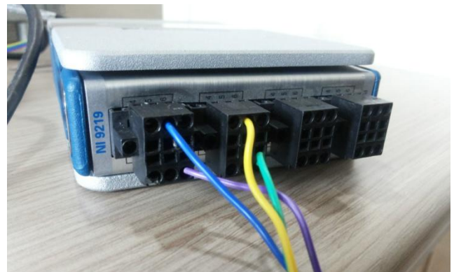
Fig.12 Wire connections to NI 9219 module.
