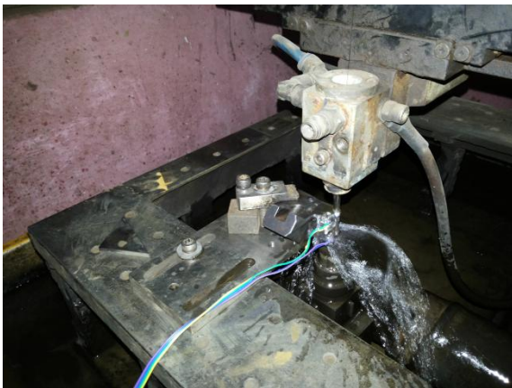
Fig.14 Shifter under cutting process
