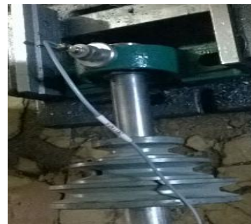
V. ACTUAL EXPERIMENTAL SETUP WITH THE ACCELEROMETER USED
