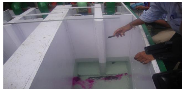
Fig.3 Observation of the Flow pattern Dye Injection Test
