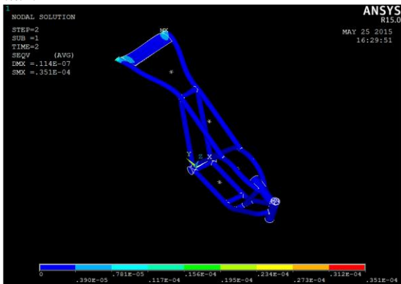
Fig. 11 Stress distribution for titanium chassis
