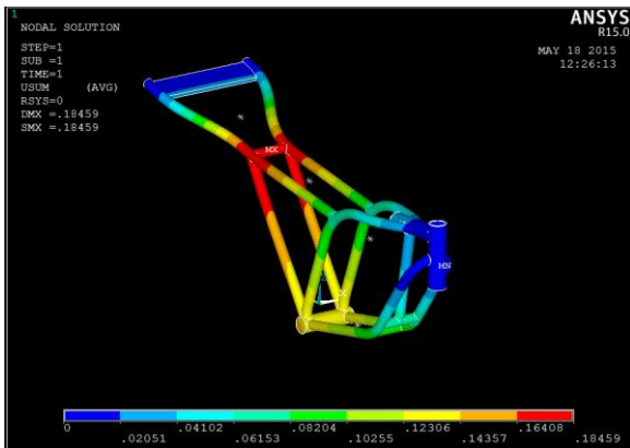
Fig. 10 Displacement pattern for carbon fibre chassis
