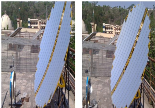
Fig 2 : Scheffler Collector System For Experimentation with (L to R ) Cylindrical and Conical Receiver at MIT,Pune
