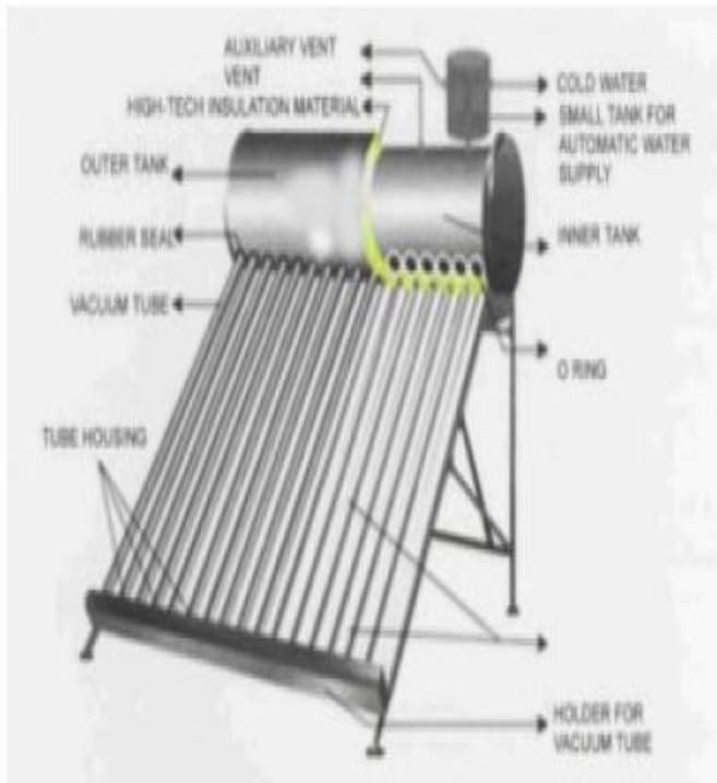
Fig.5- Evacuated tube solar water heater
