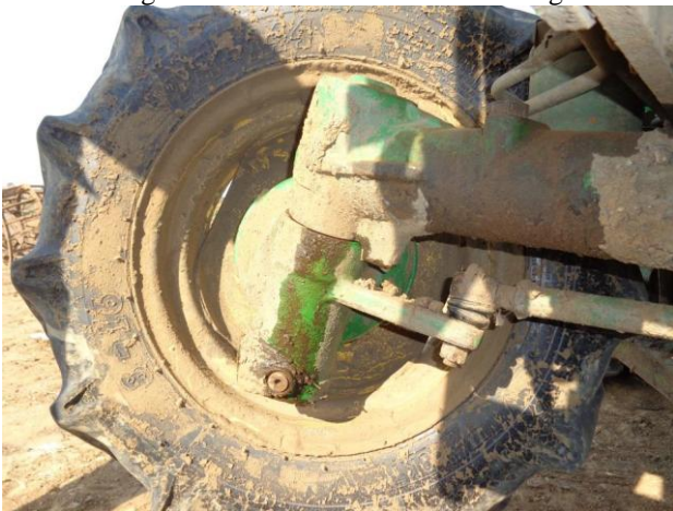
Fig.14 Field testing of axle with New Housing
