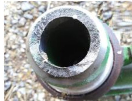
Fig .2Failed housing
