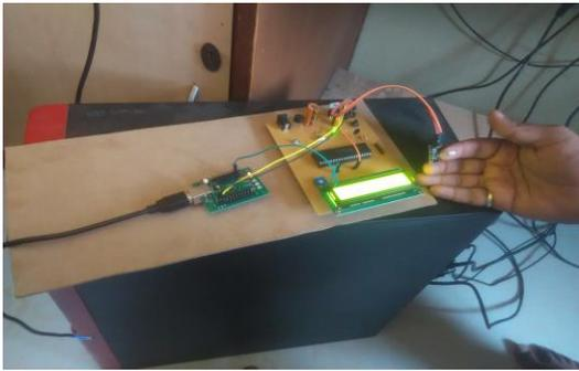
**Figure1:** Pulse sensor connected to Medical diagnostic platform
