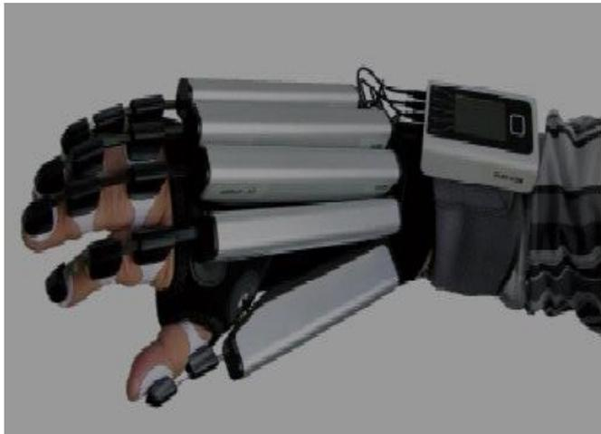
Fig 3. An example of a CPM device which uses actuators for delivering the push and pull exercises to the finger's joints
