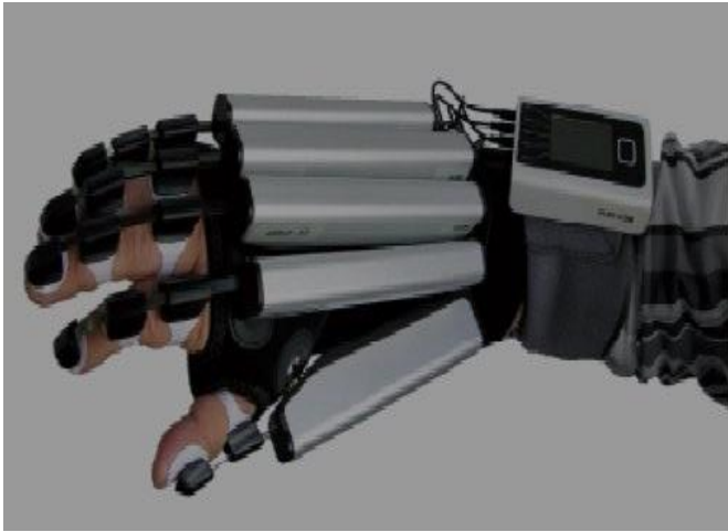
Fig 3. An example of a CPM device which uses actuators for delivering the push and pull exercises to the finger's joints
