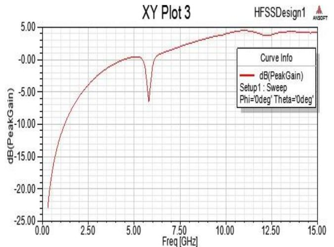
Fig.7. Gain of the proposed antenna
