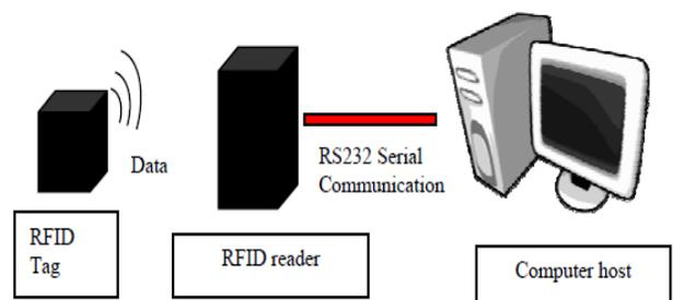
Fig. 1 Working of RFID system
