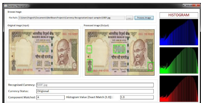
Figure 5. Front panel of software showing the given input image of currency note is "Original"
