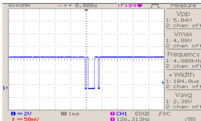
Fig 2. Serial Data for Transmitting Pc
