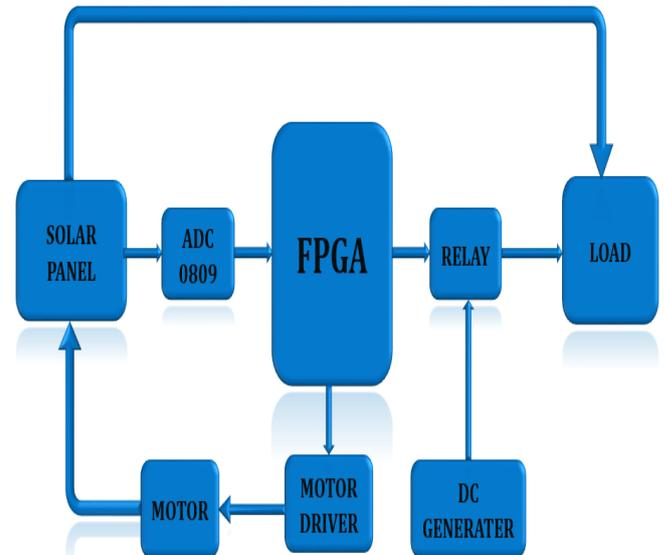
Fig 1: Block diagram of FPGA based solar tracking with backup system
