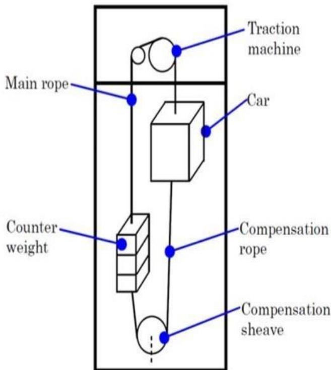
Fig.1 - schematic diagram of an elevator system
