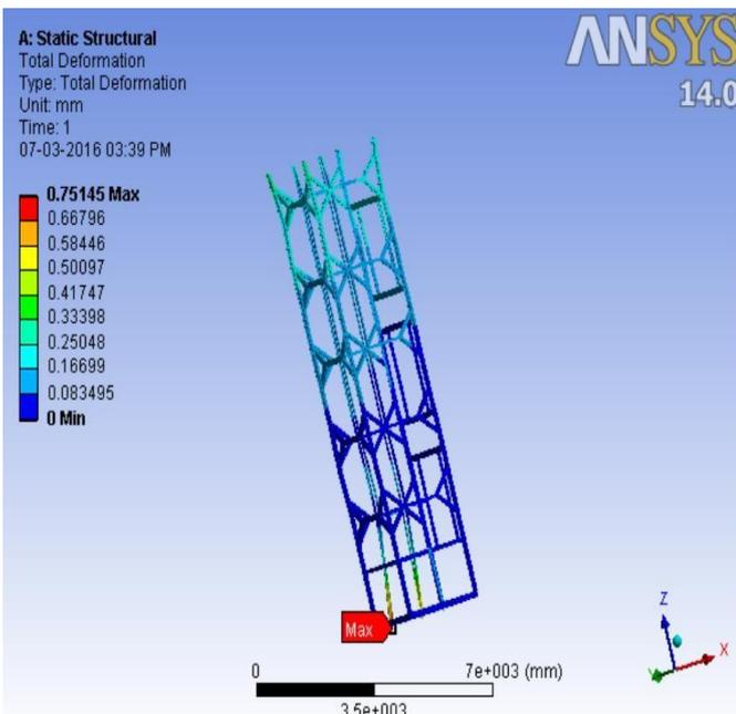
Fig 4 – simulation results showing deformation in the structure.
