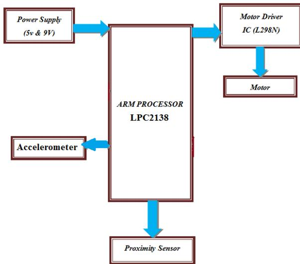
Fig 1. Block diagram of Self-Contained Localization of Small-Sized Ground Robotic Vehicle.
