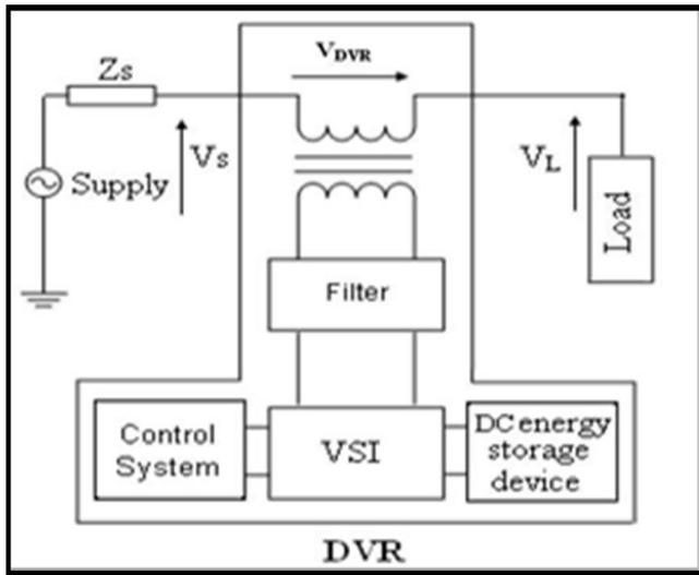
Fig. 1 Block Diagram of DVR
