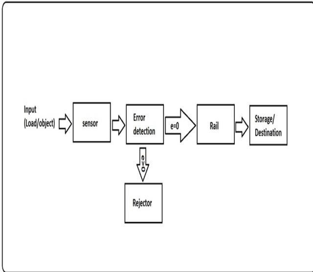
Fig. 1 Block diagram of automatic storage system
