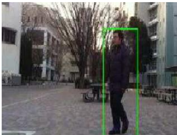
Fig. shows the simplified diagram of this detection process. FFmpeg is used only to decode the video stream. Then, the object detection function uses the decoded data to detect any moving object by using the available programming interfaces provided by Open CV. We have presented video motion detection methods, motion vector (MV) based and, using open source tools, FFmpeg and OpenCV libraries. With the existing tools, we could build moving object detection application by simply extending the video decoding functions .
