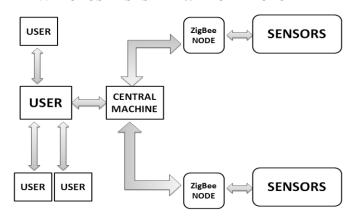
In This Sytem, Sensors Deployed in the Environment Will Monitor the Environment Continiously, If there is detection of Fire, Sensors will get tripped and will communicate with Corresponding Zigbee Node And transfer their current data to the Zigbee Node .
