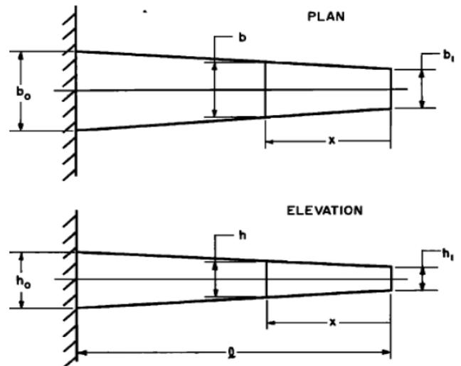
Fig.4 Plan and Elevation view of cantilever tapered beam with linearly varying width and depth
