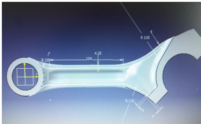
Fig.7 Connecting Rod With Extra Material
