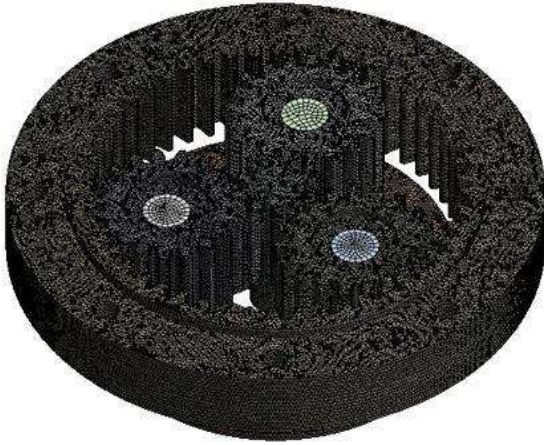
Fig.7 Meshed model of Epicyclic gear train
