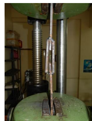
Figure 4: Specimen Prepared, Mounted and Tested on the UTM machine
