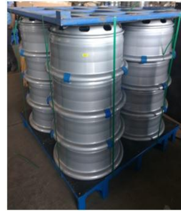
Fig. 9 Modified Packaging Scheme with Separator Clip
