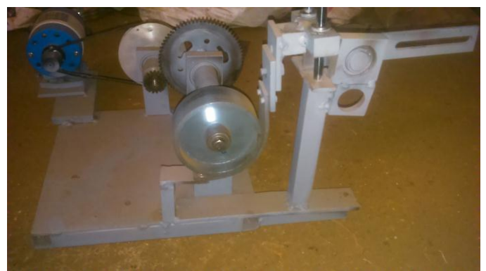
Fig.2 Test-Rig Used For Testing of Band Brakes
