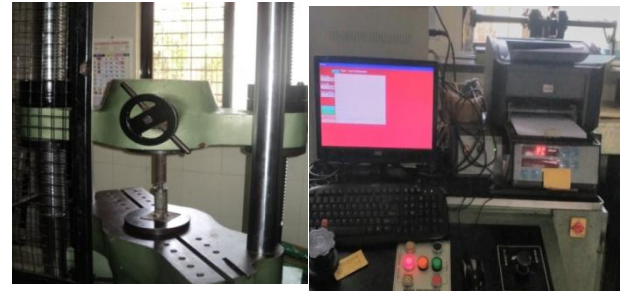
Fig.1: Compression Test of spring on UTM and display of P Vs \delta response of spring on computer screen
