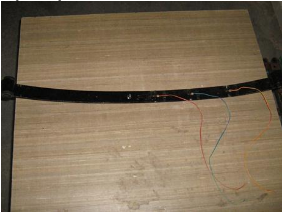
Figure: 6.2 Leaf spring with three strain gauges mounted.
