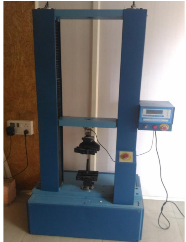
Figure 4: Pullout test machine
