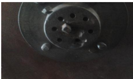
Fig 3. Shaft of the blower after drilling of holes.
