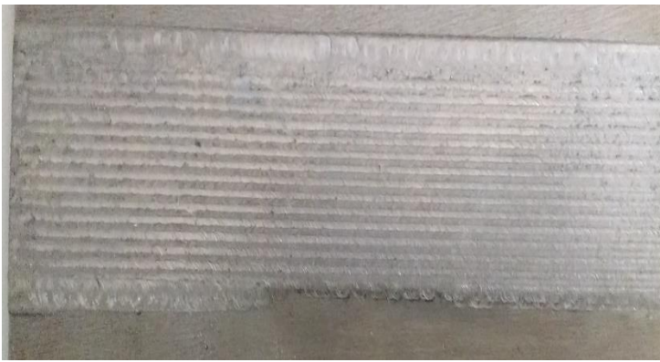
Fig.2.Friction stir plate with worktable 0.4 mm upward and tool speed 720 rpm
