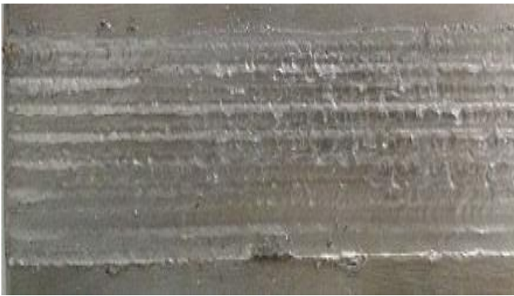
Fig.3. Friction stir plate with worktable 1.5 mm upward and tool speed 720 rpm
