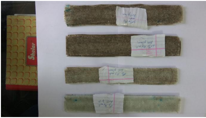
Fig10. Test Specimens of various (10%, 30%, 40%) of fly ash content and pure composite material.
