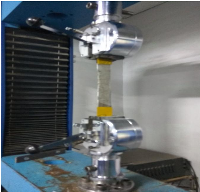
Fig11. Specimen on UTM during tensile test
