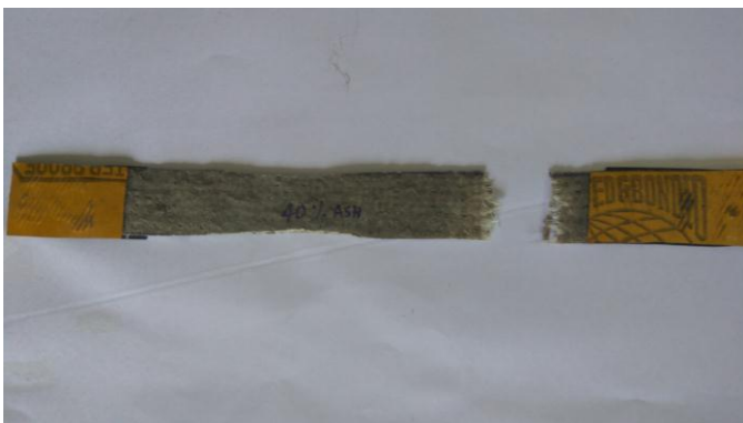
Fig12. Specimen of fly ash content of 40% after testing
