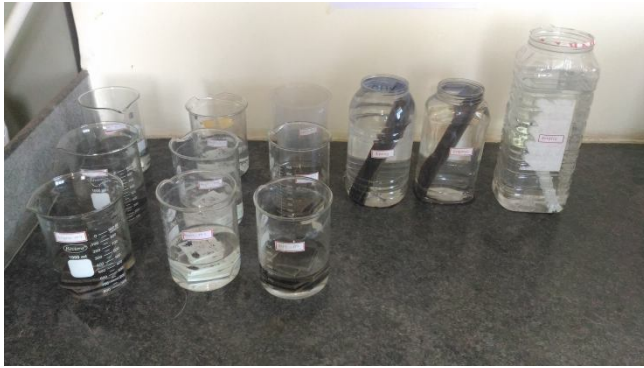
Fig. 1. Experimental set up of moisture study in jute-epoxy coated and uncoated specimen exposed to different solution media
