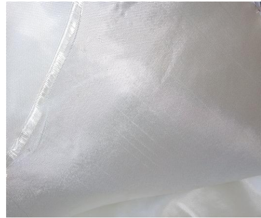
Fig. 1. Glass Fiber Cloth used for making of the Composite Laminate
