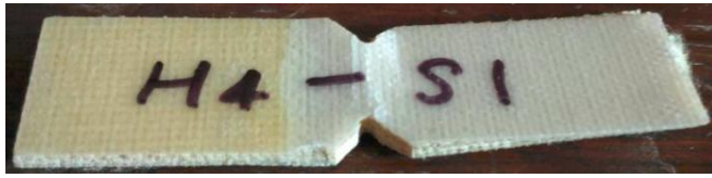
Fig. 11. Failed Shear Test Specimen
