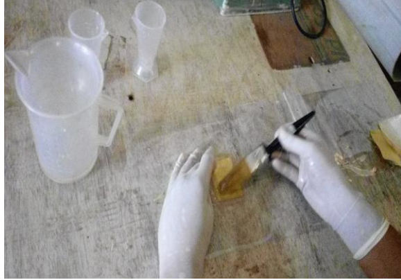
Fig. 3. Preparation of Composite Laminate Using Hand Lay-Up Process
