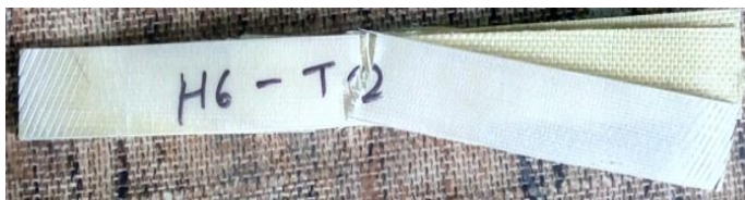
Fig. 8. Failed Tensile Specimen
