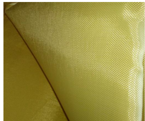
Fig. 2. Kevlar Fiber used for making the Composite Laminate
