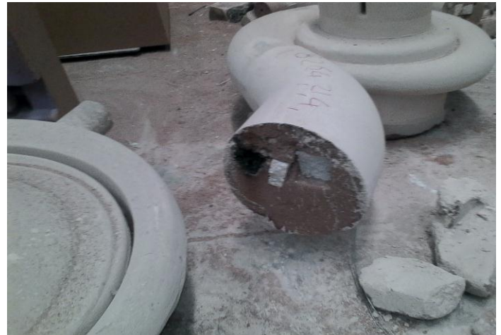
Fig E4.a (i) core with core saver for UG118294-0000
