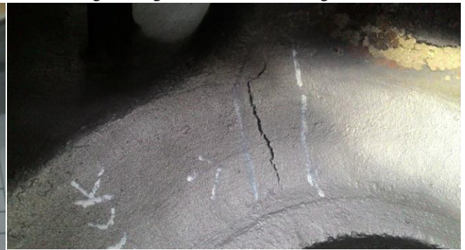
Fig E.1 .f(ii) shows the actual cracks in a casting This method is used to reveal surface discontinuities by bleed out of a colored or fluorescent dye from the flaw. The technique is based on the ability of a liquid to be drawn into a "clean" surface discontinuity by capillary action.
