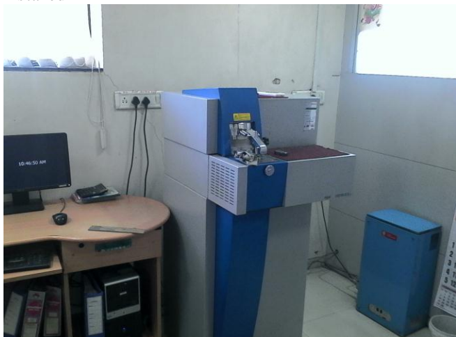
Fig E. 1. d (i) Setup used to checked the metal chemistry
