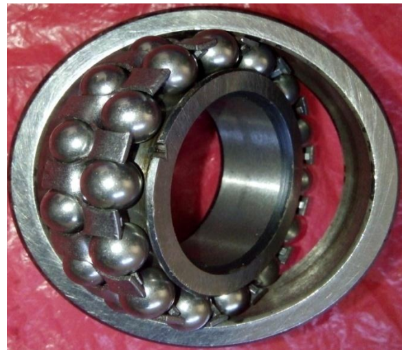
Figure 4 Fault on inner race.
