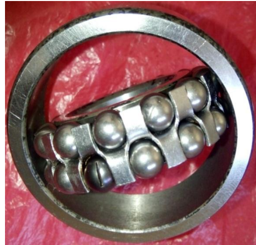
Figure 3 Fault created on ball.
