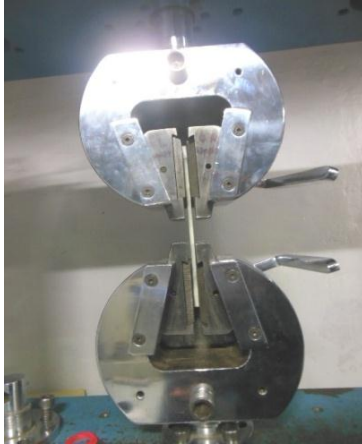
Fig. 4. Tensile test for finding material properties
