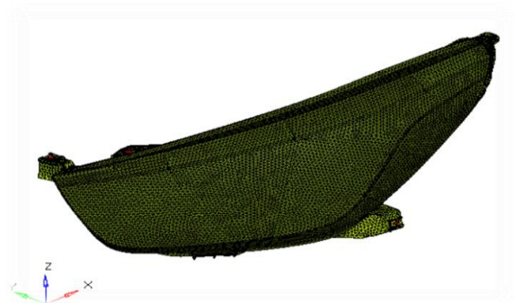
Figure 5. Headlamp meshed model using Hyper mesh
