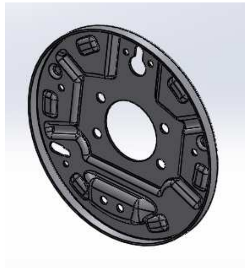
Figure 5: Backplate with Ribs, Nodes1061134, Elements 651749, Weight 7 N
