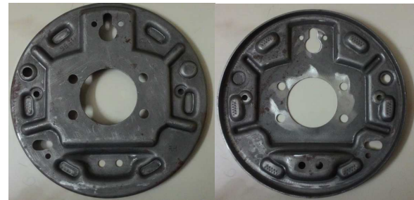
Figure 7: Backplate with design modification to increase stiffness
