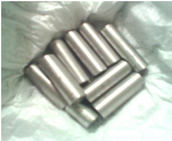
Fig.1: Babbitt Pin Manufactured for Testing
