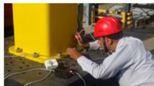
Fig. 19 a) Experimental setup for Strain measurements
